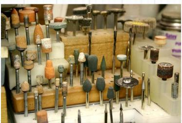
The wide variety of bits available for rotary tools makes them a must-have in the budget-friendly prototyper's workshop.
