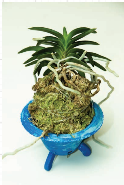
Color break on an 3D printed ABS orchid pot treated with acetone.
