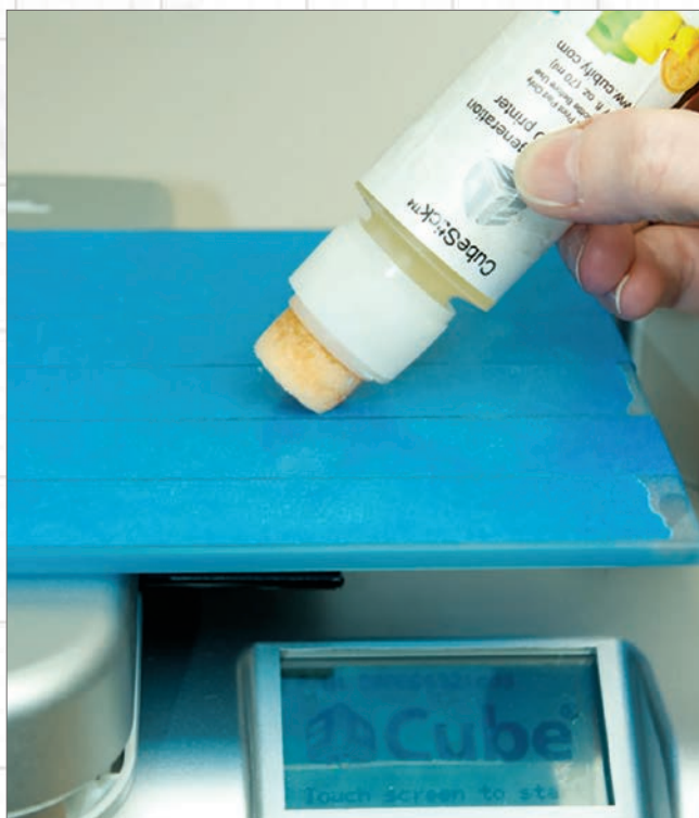
CubeStick and masking tape on the build platform helps keep prints from pulling off the print bed.
