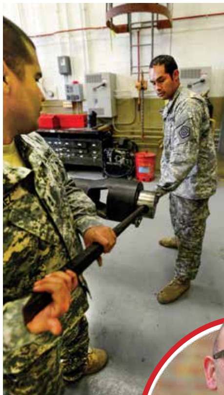
Far left: Sgt. Wesley Todd of La Porte, Indiana, checks measurements on the device he invented at the machine shop in the Combined Support Maintenance Shop in North Riverside, Illinois. Near left: Sgt. Michael Georgeff of Bourbonnais, Illinois, and Sgt. 1st Class Edgar Gomez of Oak Lawn, Illinois (facing away from camera), use Sgt. Todd's invention and a pry bar to remove the muzzle from a light-towed howitzer.
