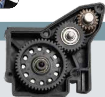
These are the inner workings of an RC car gearbox. Motor torque comes in from the shaft on the upper right and out through to the wheels from the largest gear on the bottom.
