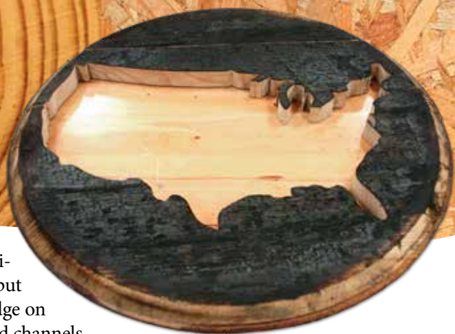
This U.S. map was waterjet cut from the lid of a used whisky barrel. The waterjet blasted through the more than 1-inch-thick wood and created a smell of vanilla and whisky.
