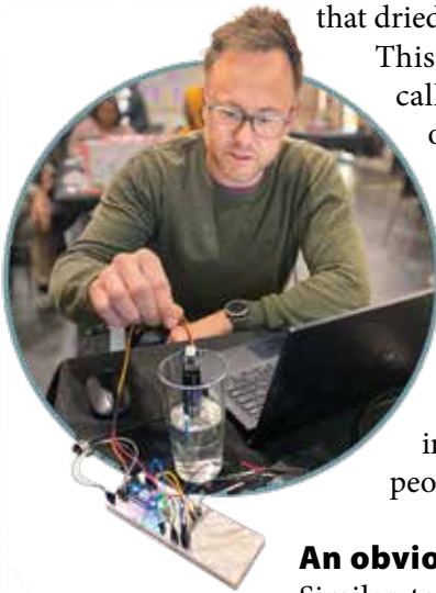
Wouter Vermeulen tests code for a moisture sensor using a Particle Argon WiFi board.
